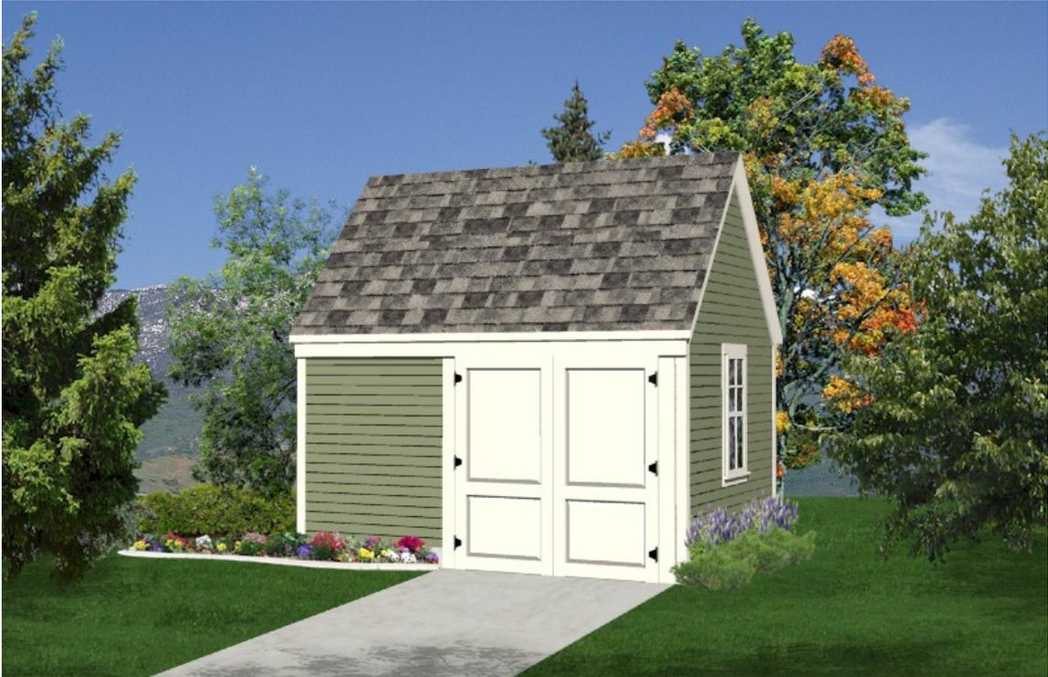
This solid, permanent 2x4 stud-frame shed, on a concrete slab foundation, has convenient lofts for additional storage.
